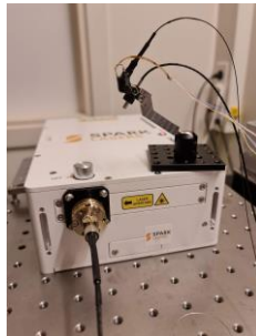
Photo of ALCOR 920-Mini2P coupled to a miniscope (taken by the "Mini2P team" at NTNU, Kavli Institute)
